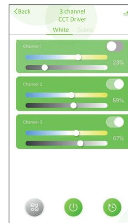
On the Smart Driver Control Menu page the lights plugged into each port of the Smart Driver are displayed in the green boxes as channels. Channel 1 controls ports 1 and 2, Channel 2 controls ports 3 and 4, and Channel 3 controls ports 5 and 6. Each channel can be controlled individually by using the slider bars and buttons.
