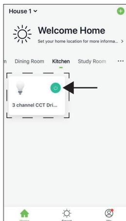
From the home page you can turn the Smart Driver on/off using the power icon on the side of the Smart Driver tab, or you can press the Smart Driver box to access the Control Menu.
