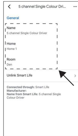
From here you will be able to change the name of the device, reassign the device to a different home and reassign the device to a different room.
