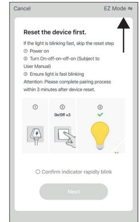
Once the lights are flashing quickly, return to the Sensio app and check that it says 'EZ Mode' in the top right corner of the screen.
