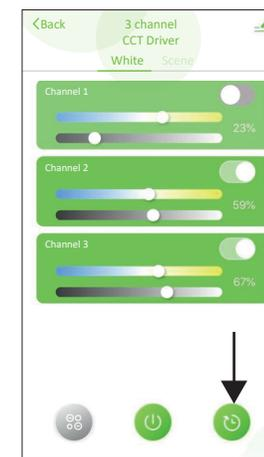
Every channel can be turned on/off as a group by pressing the power button located at the bottom centre of the page and channel names can be modified by pressing the channel titles in the top left of the green boxes.
