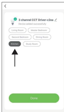
Once connected, you have the option to assign the Smart Driver to a room and you can also edit the name of the Smart Driver by pressing the pencil icon next to it.
