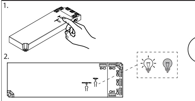
At this stage you will need to press the 'Wifi pairing' button on the top of the smart driver 4 times and then wait 10 seconds until the lights begin to flash rapidly (approximately on/off once per second). If the lights are flashing slowly, press the button a further 4 times until they begin to flash quickly.
