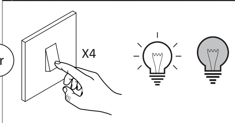
At this stage you will need to switch the Smart Driver off and on four times, pausing for 2-4 seconds between each flick of the switch. After approximately 10 seconds, the lights should begin to flash rapidly (approximately on/off once per second). If the lights are flashing slowly, flick the switch a further 3.5 times until they begin to flash quickly. If they do not, turn the lights off for 30 seconds and try again.
