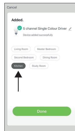
Once connected, you have the option to assign the Smart Driver to a room and you can also edit the name of the Smart Driver by pressing the pencil icon next to it. **Caution:** If you are planning to connect your smart driver to a smart device for voice commands, we do not advise changing the Smart Driver name. Instead we recommend that you change the driver name in the Alexa or Google Home App. For more information see pages 9 and 12.
