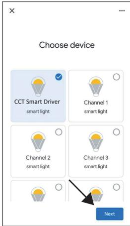
At this stage you will need to set up each device individually. To do this, press the device you want to set up so it is highlighted in blue and then press 'Next'.
