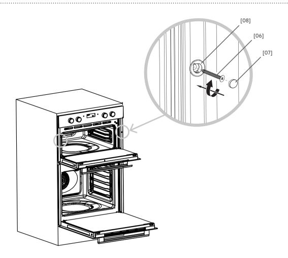
EN Once the oven has been lifted into place inside the appliance housing, locate the two holes in the casing of the oven and fix it into place using [06], [07] and [08].
