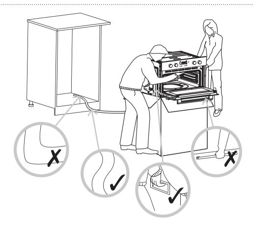
EN Important: Do not lift the appliance by the door handle to avoid potential damage to the glass and hinges.
