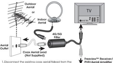
Disconnect the existing coax aerial flylead from the ANT IN socket on the back of your TV or set top box and connect it to the socket on your 4G filter.
