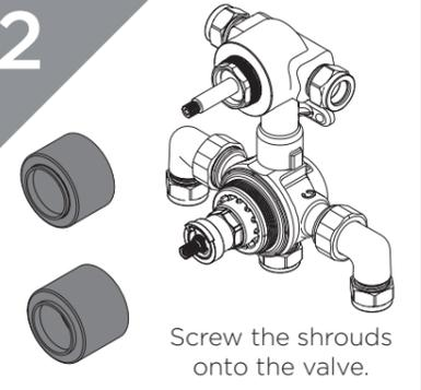
Screw the shrouds onto the valve.
