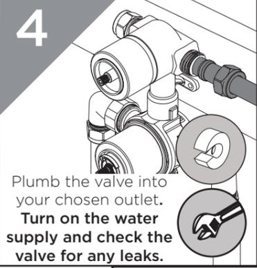
Plumb the valve into your chosen outlet. **Turn on the water supply and check the valve for any leaks.**
