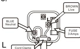
**WARNING:** Never connect live or neutral wires to the earth terminal of the plug.
